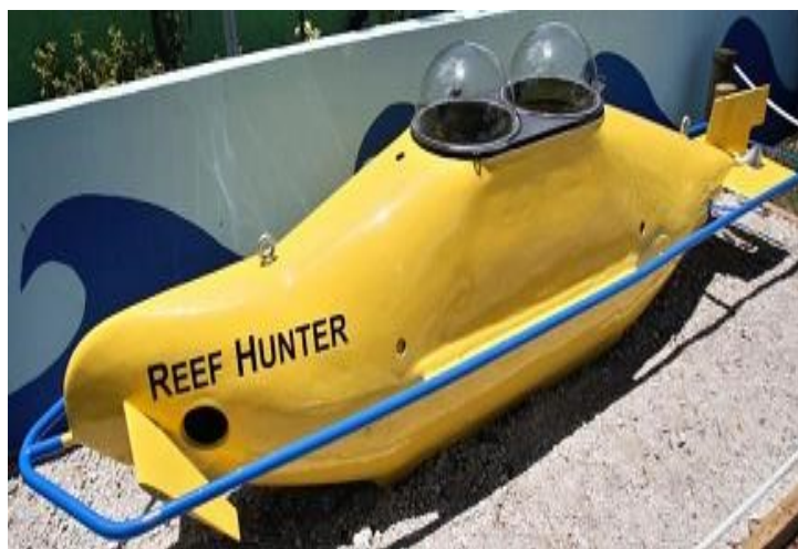
Fig. 2: The late 1950's Perry Cubmarine ; a plywood and fibreglass two person submersible that could reach a depth of about 50 metres for observational missions.
